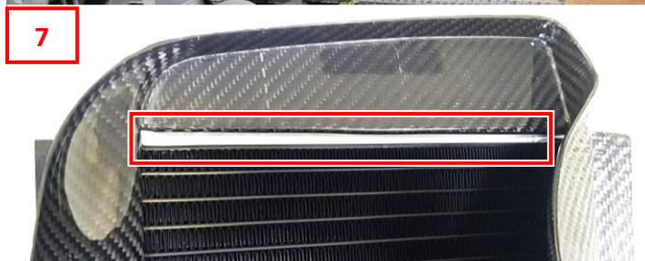
*Connect the WT air duct 002001064 to the WT intercooler 001001125 and the WT air duct 002001063 to the WT intercooler 001001126.*
